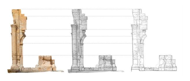
$Puc.\ 3.\ \Phi acad\ nunohob\ D\ u\ E.\ Перевод\ opmoфomochumкa\ modenu\ b\ чертеж$   $Fig.\ 3.\ Façade\ of\ pylons\ D\ and\ E.\ Converting\ the\ orthophoto\ from\ the\ model\ into\ a\ drawing$
